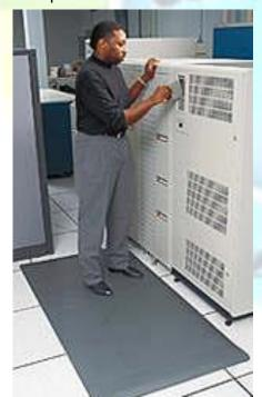
damaged by simply laying it on a bench top. For this reason, you should have an ESD mat in addition to an ESD strap. This mat drains excess charge away from any item coming in contact with it. ESD mats are also sold as mouse/keyboard pads to prevent ESD charges from interfering with the operation of the computer. ESD charges can cause a computer to hang, reboot or generally cause problems.
