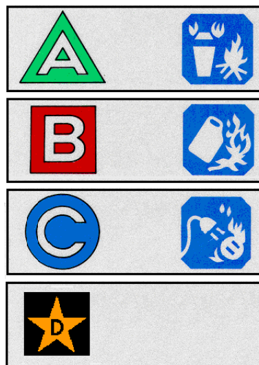
Figure 6: Pictographs to label a fire extinguisher
