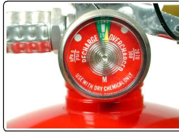
Figure 3: Fire extinguisher gauge
